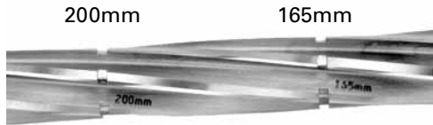
Figure 4 Straight Reamer Depth Markings
